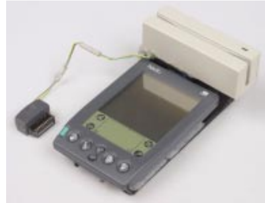
Skimmer attached to Palm Pilot™ for data downloading.
